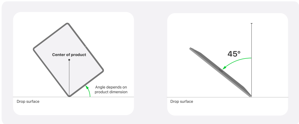
Drop orientations for "lower right edge" (left) and "lower right front corner" (right).
