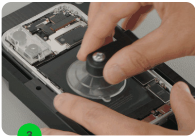
Lift the battery from the enclosure using a suction cup.
